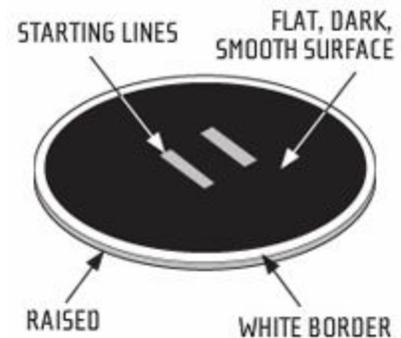
LEGO Sumo takes place in a circular ring four feet (122 cm) in diameter with a two-inch (5 cm) white border along the ring's perimeter. The surface of the ring is smooth plywood (painted black) and is about one and one half inches (3.8 cm) above ground level. The raised platform helps to determine when a robot has "fallen off" (generally determined by the robot touching the ground outside the ring, but left up to the judges discretion).
